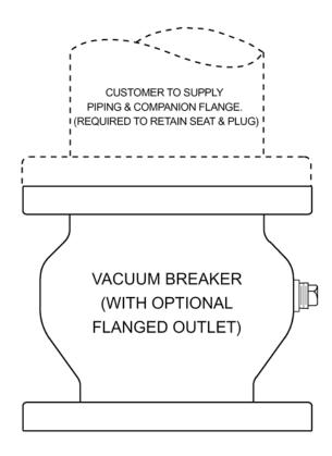
FIGURE 2. VACUUM BREAKER WITH OPTIONAL FLANGE
