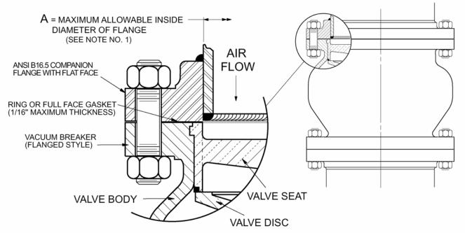
NOTE NO. 1 - THE MATING COMPANION FLANGE I.D. MUST OVERLAP THE VALVE SEAT. THIS IS REQUIRED TO PROVIDE PROPER SEAT RETENTION.
