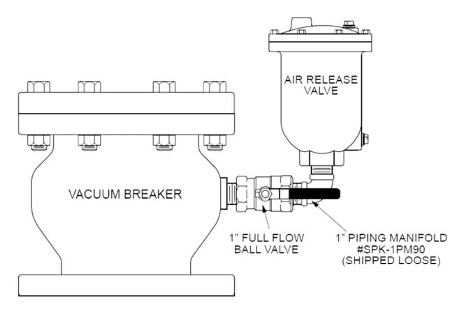
FIGURE 3. VACUUM BREAKER WITH OPTIONAL AIR RELEASE VALVE
