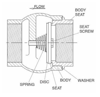
FIGURE 1. THREADED SILENT CHECK VALVE
